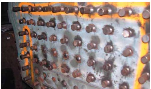
The hard work has started. Probably hard to see, but some of the stays on the fourth row down have been cut and rivetted. As also are some around the firehole ring. Hats off to those doing this unenviable task!
