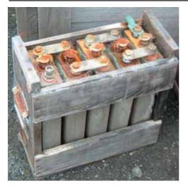
Can anyone give a story as to the background and purpose of these type of batteries? We have two here and so far, no one has been able to come up with an answer as to the purpose attached to them. You will note that there are only five cells. That would nominally suggest, 5x1.2v=6v, which would have to be a very marginal 6v at that. The cases have been very well made and they would be about 14/16 inches tall.
